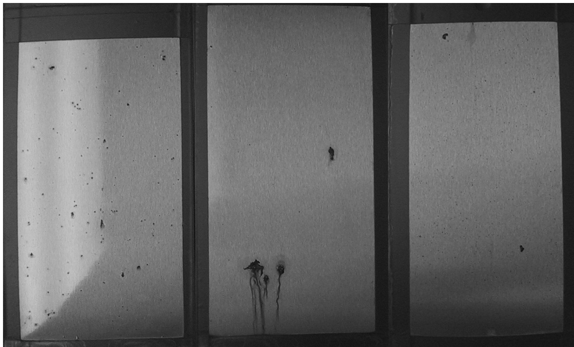
Figure 2 – Corrosion Resistance at 312 Hours Salt Fog Exposure
