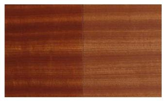
Left: first coat with UV-PUD 4. Right first coat with UV-PUD 1
