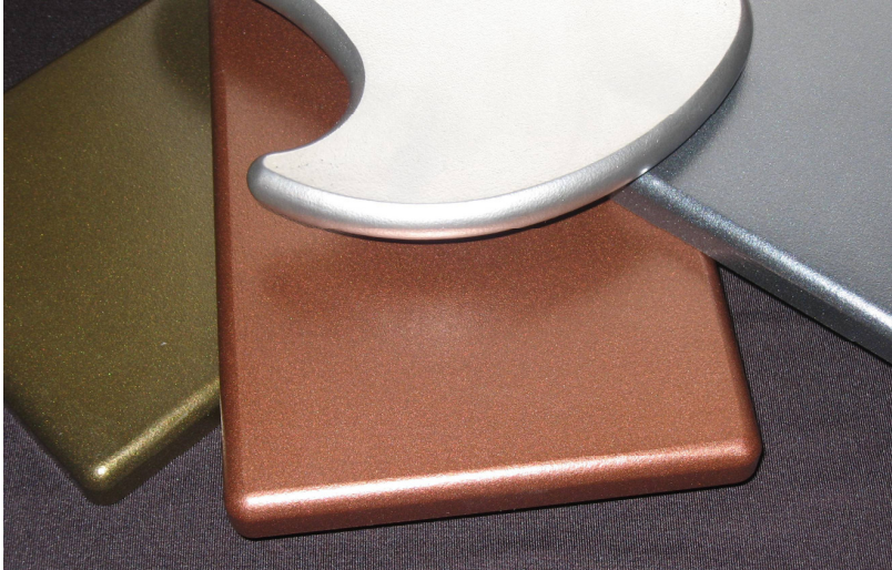
Figure 1: UV cured metallic powder coatings on MDF substrate, Gold, Bronze, Dark Silver and Bright Silver
