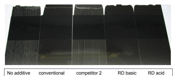
*Figure 8.0 Photograph of cured Special Black 250 flexographic formulation on Leneta Black and white card*
