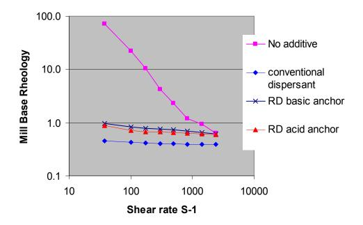
Figure 3.0 Rheology flow curve of 30wt% dispersion of Regal 400R pigment
