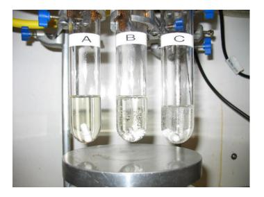
Figure 6.0 Radical polymerisation of butyl acrylate
