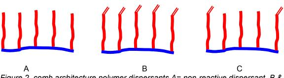
*Figure 2. comb architecture polymer dispersants A= non-reactive dispersant, B & C reactive dispersants.*
