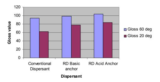
Figure 5.0 Gloss measurement of Regal 400R based cured inks.
