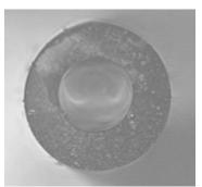
Figure 2. A 500µm Upjacketed Fiber with the Bufferlite<sup>TM</sup> DU-3038 series a single coat over a standard coated optical fiber .
