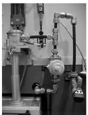
Figure 3. Modified Color Machine for High Capacity Upjacketing Process
