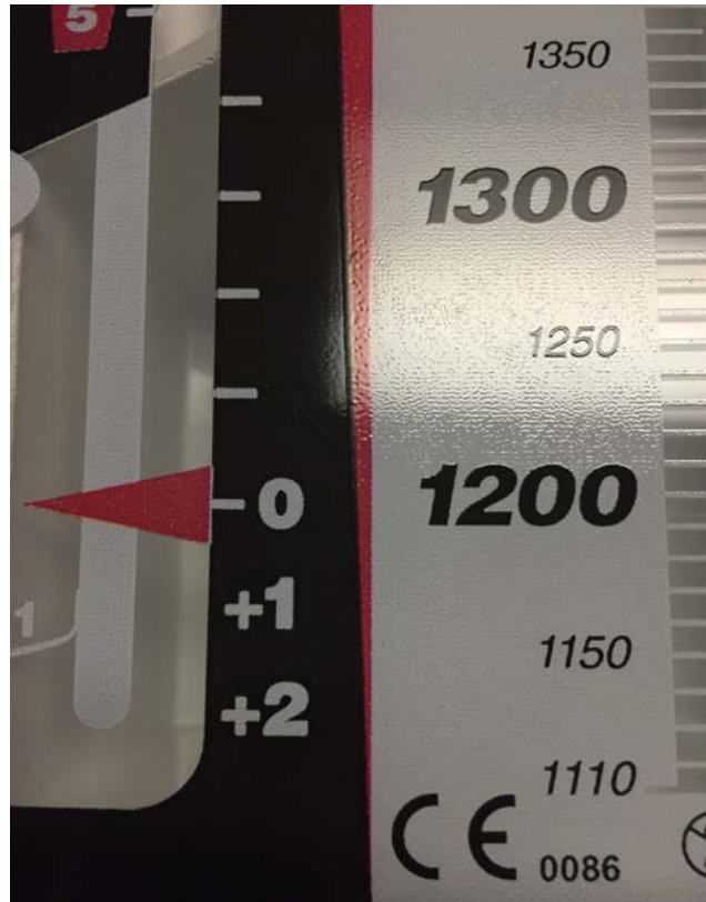
Figure 1 - Example of Image Quality Achieved in Early Samples (Photo from Full Scale System Print) that Highlights the Graduation Marks and General Print Quality
