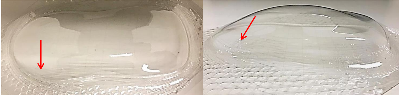
Figure I: Formed part with cracking and delamination in the areas with a higher degree of thinning.
