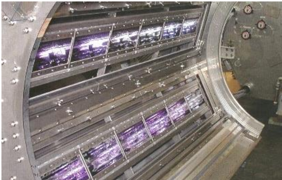
Picture 2. 2x6 Microwave systems in a closed chamber (Courtesy of Heraeus Noblelight North America)
