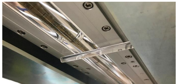
Picture 3. Close-up of ICAD™ rod in front of UV LED Array
