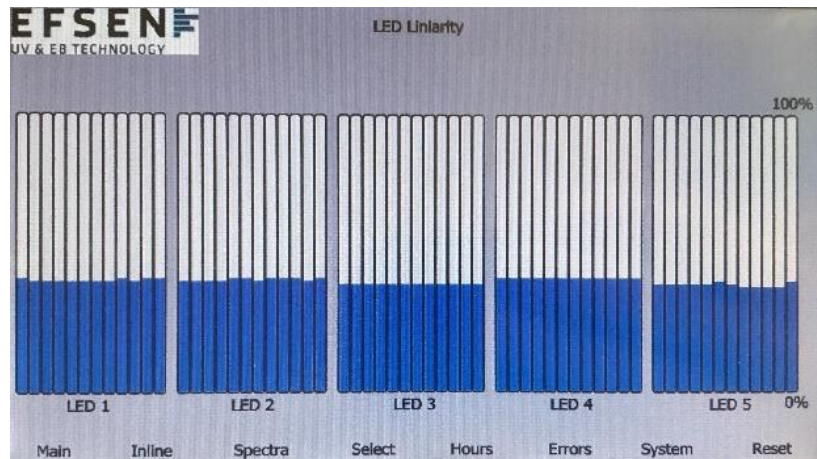
Figure 2 measurement of 5 pcs AC8300-395 UV LED heads after “calibration” of heads
