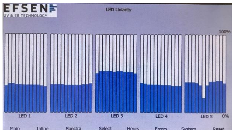
Figure 1 measurement of 5 pcs AC8300-395 UV LED heads.
