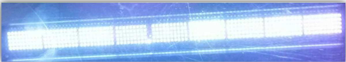
Picture 1. Close-up of 9 UV LED sections with one (no.4) being faulty (Courtesy of Excelitas/OmniCure)
