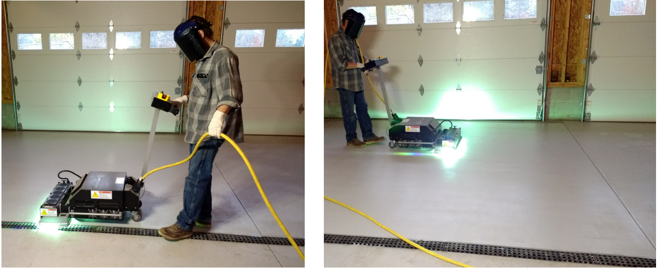
Figure 2. Quick Cure Of Biobased Industrial Floor Coating With A UV Cure Floor Machine
