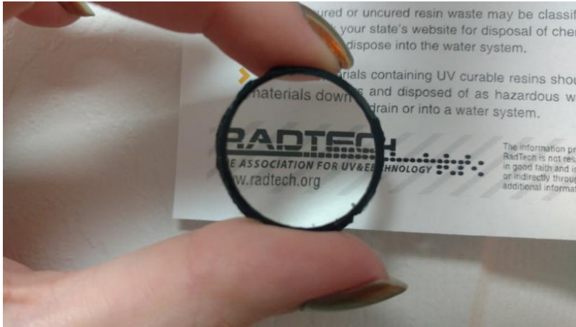
Figure 7: CPS 2 shown in a flat configuration. CPS 2 is a crown material and has a refractive index of 1.54 and an Abbe number of 50.
