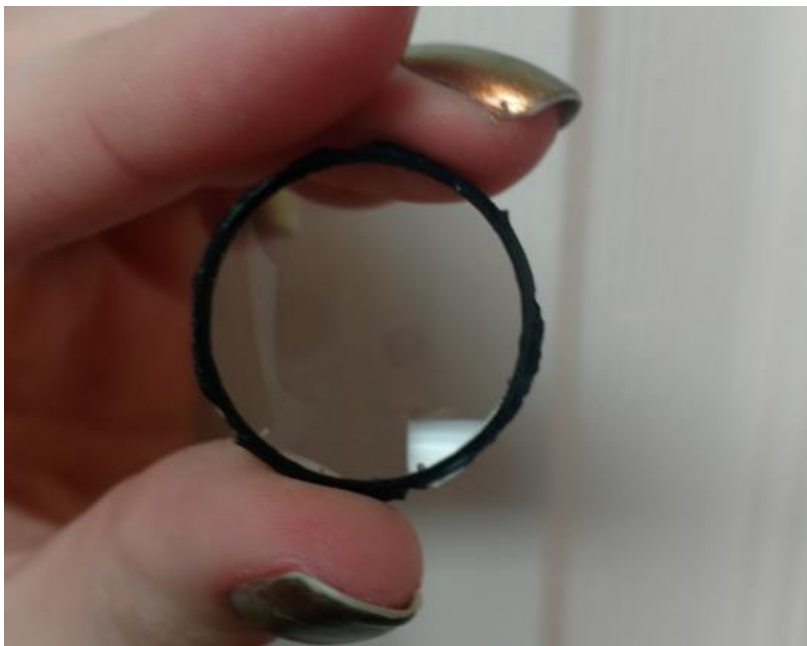
Figure 8: CPS 2 shown in a flat configuration. CPS 2 is a crown material and has a refractive index of 1.54 and an Abbe number of 50.
