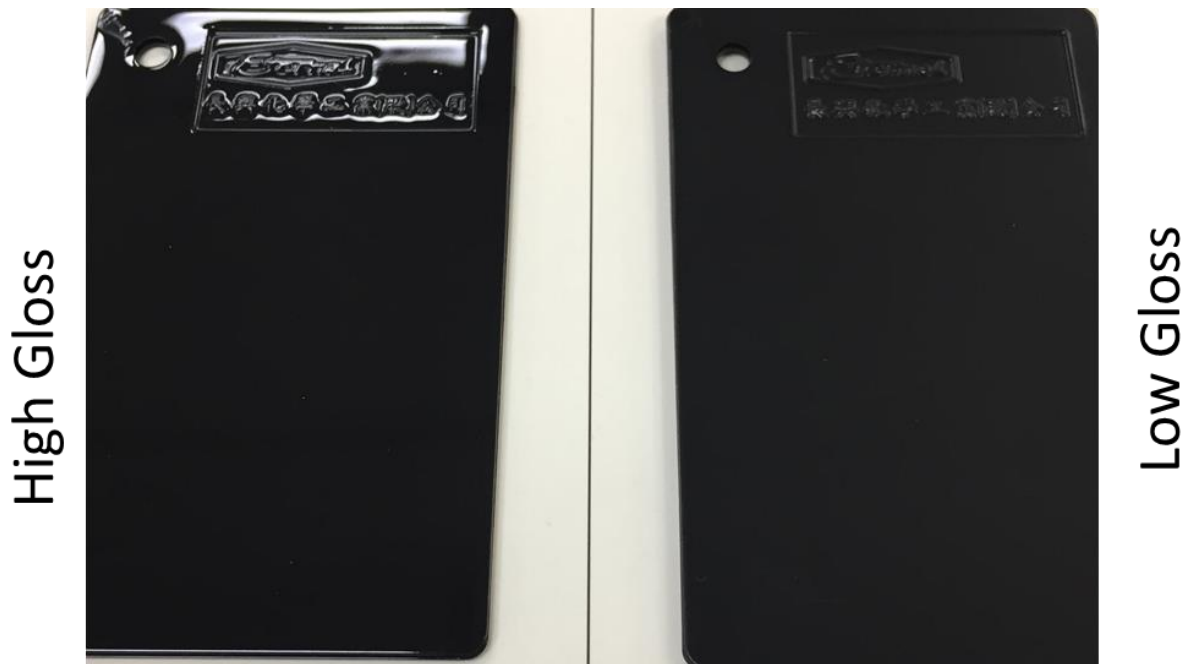
Figure 5. Single layer coatings on ABS. The pictures are taken simultaneously, i.e., under the same light.
