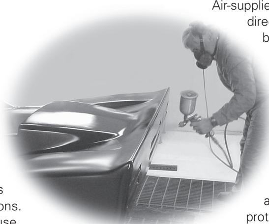
Air-supplied respirators deliver fresh air directly to the worker and should be used when air quality is unknown, when applying coatings that contain isocyanates or highly reactive catalysts, and when applying solvent-based paints in confined areas. Consult the MSDS and labels for recommendations on the appropriate respiratory protection to be used when components are mixed together and applied in multiple-component coatings systems.
