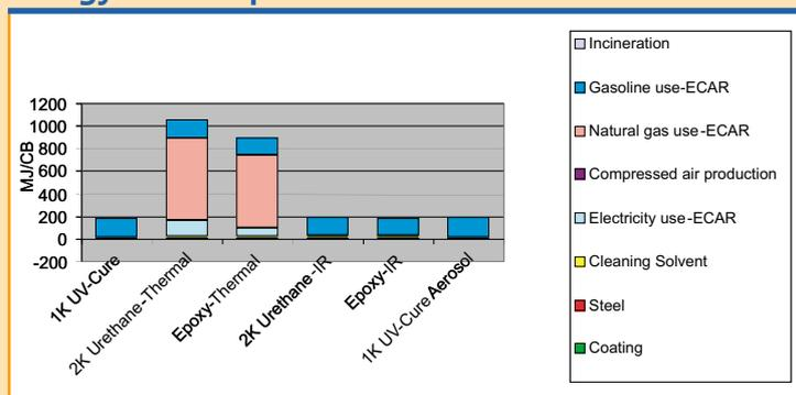
processes, which consume large quantities of natural gas and result in correspondingly higher environmental impact and utility cost. This characteristic is also the reason for the high resource consumption of the thermally cured coatings.
