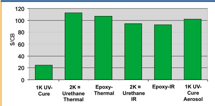
curing processes they have less overall environmental impact and lower costs than the thermally cured coatings. The UV-cured coating in aerosol cans has similar environmental impact to the non-aerosol product; however, the higher material cost results in lower eco-efficiency.
