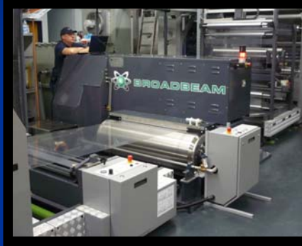
Low voltage EB system on web offset press
