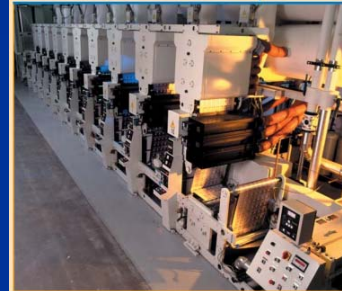
Interstation UV installation on a flexo press
